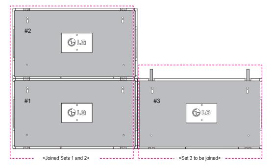
Minimize the space between the sides of the sets using the U-shaped fixture.
